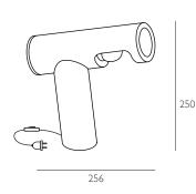
BODY limestone and brass CABLE 3000 mm with hand switch and Euro-plug DIMENSIONS (mm) 256L x 90W x 250H
