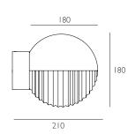
FRAME steel, powder coated SHADE handblown glass, coloured DIMENSIONS (mm) 210 L × 180 W × 180 H
